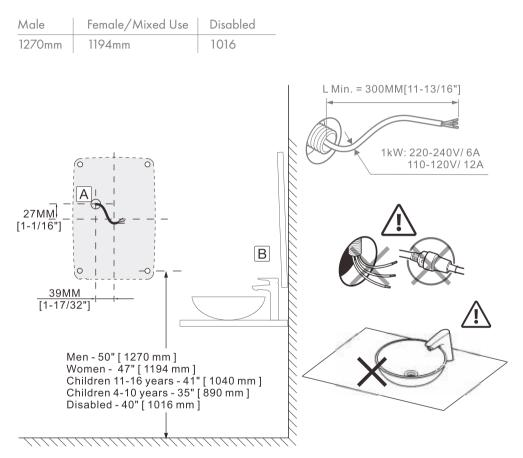
It is recommended to avoid installation of dryer near high reflective objects (mirror, stainless steel washbasins, etc.) in order to avoid faulty function of the presence sensor.
